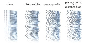
**Figure 13:** Simulated noise of a Velodyne HDL-64E scanner. Here we show an example of the two noise types introduced by this scanner: distance bias (db) adds an error to the depth of scan lines, while ray noise (rn) adds an error to the depth of each point. Note that the points in the ground truth (left) are not distributed uniformly, so we use the distance of each point to the surface as error measure for experiments with this dataset.
