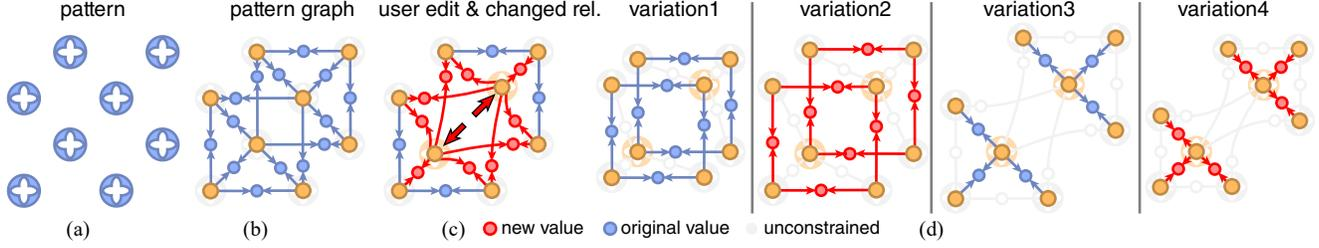
**Figure 6:** Generating pattern variations. The structure of the pattern in (a) is captured by the pattern graph in (b). For clarity, each blue relationship represents one centroid distance and one centroid direction relationship. A user edit of the two central elements (c) causes some relationships change (red). Variations can be generated by fixing relationships to their new or original values (red and blue, respectively), or leaving them unconstrained (grey).
