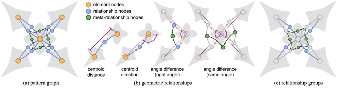
**Figure 5:** The pattern graph describes the element arrangement of a pattern. (b) Pairs of elements are related by geometric relationships. Relationship values can in turn be related by meta-relationships. (a) These relationships form a directed graph. (c) Relationship groups describe repeating structures in the graph.
