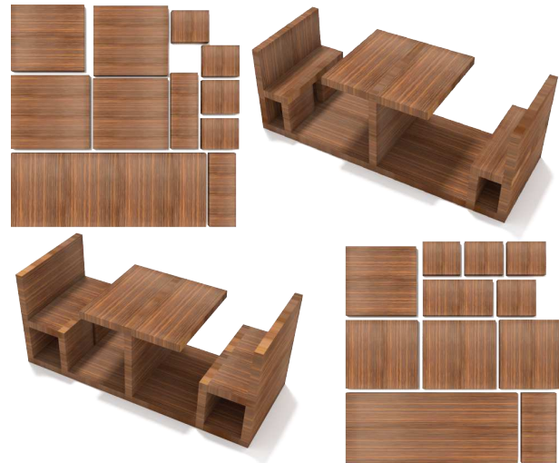
Fig. 16. Designing a chair with two chairs and a platform from a single master board. Top row shows the original design (11% wastage), while the bottom row shows the final design (4% wastage). 10-15% less wastage.
