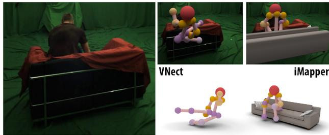
Fig. 9. **Comparison with VNect.** State-of-the-art 3D human pose detection from monocular video VNect [Mehta et al. 2017b] breaks down in regions of occlusion (VNect was not designed to handle occlusions), while iMAPPER continues to produce plausible results because of explicit occlusion detection and handling. Bottom row shows the recovered human pose from another camera angle for better visibility.
