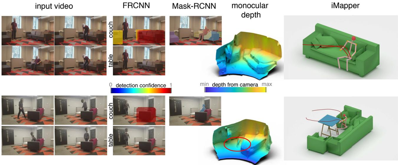
Fig. 6. **Object detection comparison.** Qualitative comparisons to state-of-the-art object detection methods. Note that FRCNN and Mask-RCNN both produce only 2D image-space segments. iMAPPER synthesizes 3D scenes that plausibly match the video, even in sequences where the objects and the human performance are occluded. Encircled in red in the bottom depth map are the typical errors near depth discontinuities obtained from image depth estimators.
