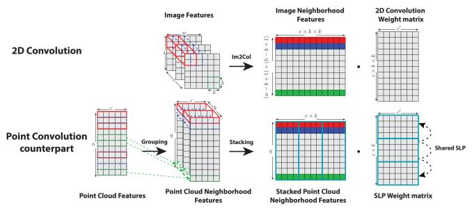
Figure 2. Analogy between 2D convolution and its point cloud counterpart. In both cases, the layer operates in two steps: (i) neighborhood exposure and (ii) matrix multiplication. 2D image convolution amounts to forming a  $K^2$  tensor in memory when performing  $K \times K$  filtering and then implementing a convolution as matrix multiplication.
