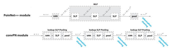
Figure 3. Comparison of a PointNet++ module with our convPN module. The convPN module replaces the MLP with its pooling layer by a sequence of SLP-Pooling modules which has two benefits (i) memory savings as the layer activations are saved only through the pooled features and (ii) better information flow as it increases the frequency at which neighbors share information.
