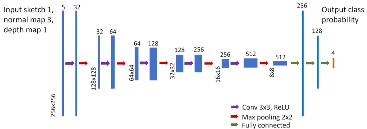
Figure 1. **The network structure for operation classification.** The input contains the sketch and context maps, and the output is the vector of probabilities for 4 types of operations.
