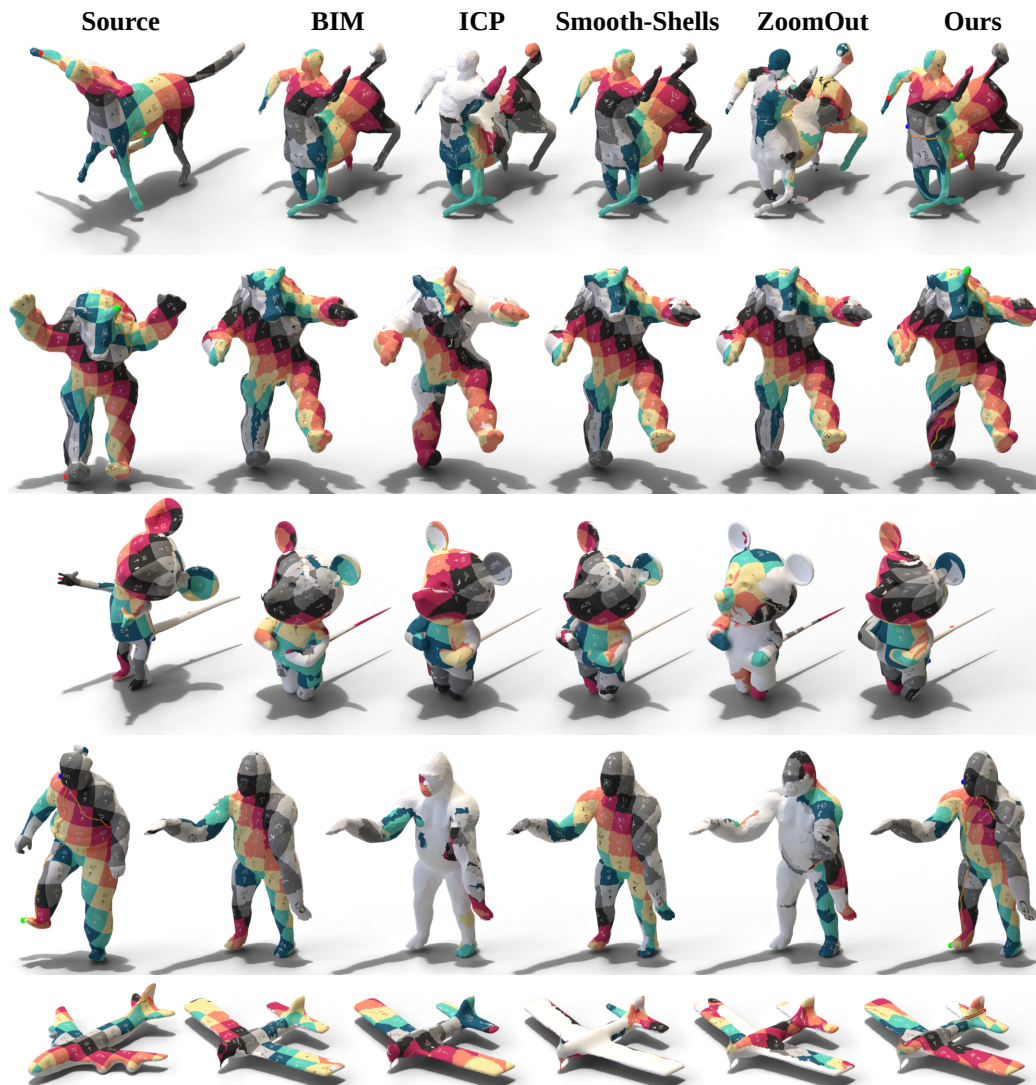
Figure 4.7: Comparisons. Left-to-right: Source model, results using BIM [114], ICP, Smooth-shells [103], ZoomOut [166], and Ours. Although geometric methods produce good maps, they often yield discontinuous maps, e.g., see the wings of planes. Ours explicitly encourages continuity and bijectivity. Coloured landmarks and paths show automatically selected cones and cuts by our method. Note that our maps are continuous across the cut seams. No explicit energy term is used to encourage isometric maps.
