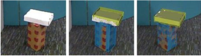
Figure 6: The initial cuboids (middle) are adjusted to better align the original image edges in the RGBD data (left) to produce refined cuboid candidates (right).
