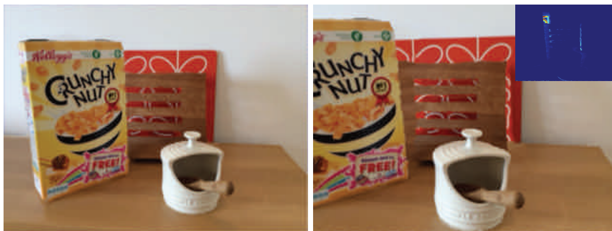
Figure 1: A single RGB-D image (left) is used to create a novel view for a parallax photograph revealing occluded regions (right) with a corresponding degradation model (inset: red and blue respectively indicate higher and lower degradation).
