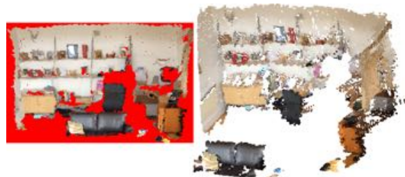
Figure 3: Example RGB-D input: Point cloud rendered from original camera pose (left) showing large regions of missing depth information labeled in red. When rendered from a different camera pose (right) the point cloud reveals many points have mislabeled depth values. The coarseness of the data emphasizes the need for decomposing the scene into geometric proxies.
