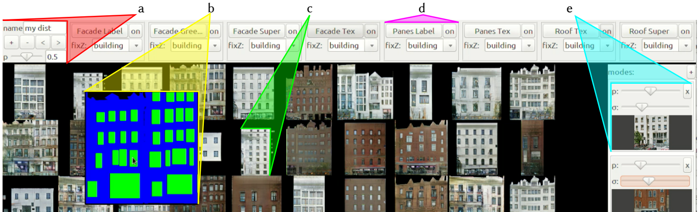
Fig. 12. The distribution designer UI (see supplemental video). Given a style distribution (a), the system continuously shows evaluations of that distribution (c). By clicking on an image, the user can see the network inputs (b). Different networks can be selected (d). The style distribution for any network is a Gaussian mixture model that may have multiple modes (e), the mean of which is given by an exemplar image.
