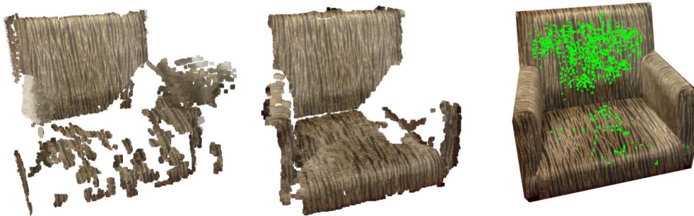
Figure 3.9: Classic dense reconstruction (left) and dense reconstruction based on our post-boosting step (middle) using the chair scene from Figure 3.6. Our pre- and post-boosting methods (right, rendered with green dots) enables the reconstruction of larger areas of the input images.
