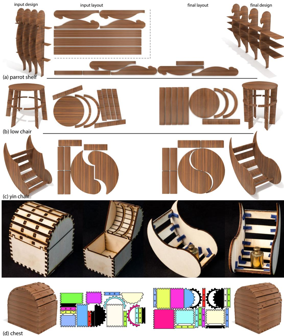
**Figure 5.16:** Curved designs. Designs created using our system. Each design is shown with initial shape, starting layout, optimised layout and final design. (a) is a constrained model while (b)-(d) are parametric models. The fourth row shows the fabricated models of the chest (left) and yin chair (right).
