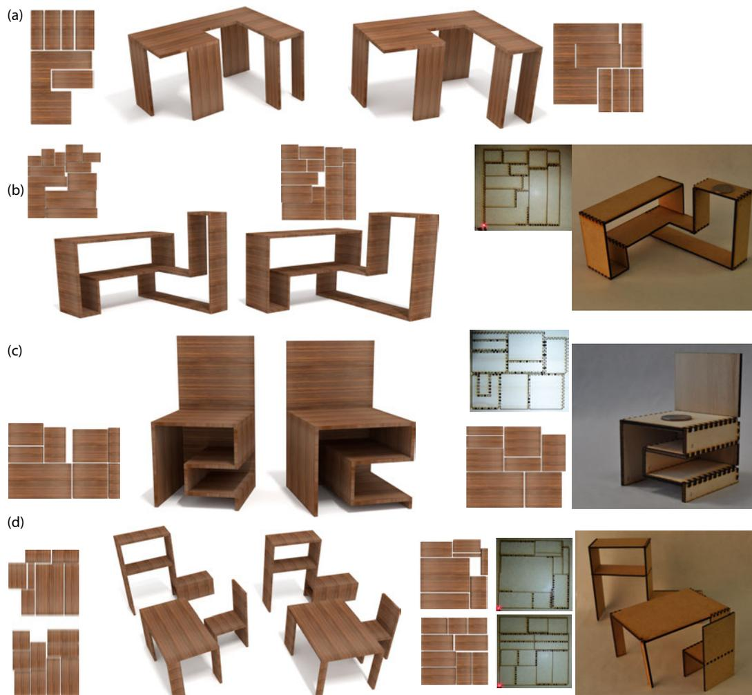
**Figure 5.17:** Fabricated examples. *Various material-driven design and fabrication examples. In each row, we show initial design (with material space layout inset), optimised design result (with material space layout inset), along with final cut-out assembled model. In (d), two master boards are used for the large design. Note that the design changes are often subtle, but still lead to significant improvement in material usage.*
