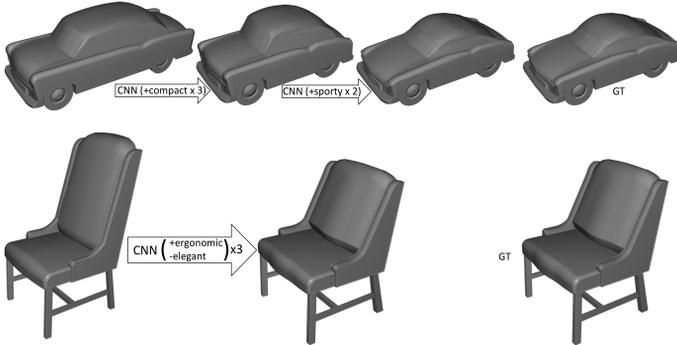
**Fig. 2.** Top: Activation of different semantic deformation indicators in successive order, Bottom: Activation of different semantic deformation indicators together.
