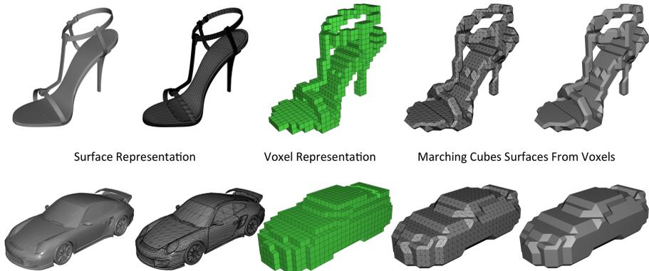
**Fig. 5.** Voxel and marching cubes surface representation examples. Note the low quality of the marching cubes reconstruction due to the low voxel resolution.
