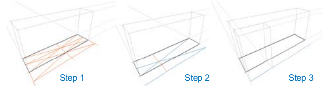
Figure 9: Guide lifetime. Guides first appear in orange (left). In subsequent steps guides that are no longer required are removed, while those that are to be reused are marked in blue (middle, right).
