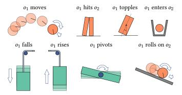
Fig. 5. **Event types.** The above events are supported in our implementation. Each event's condition  $c_e(t)$  is a function of the spatial transform (and corresponding time derivative) of the target object(s) at time t. Events may also have a negated version (e.g., ' $o_1$  stops' being equivalent to ' $o_1$  does not move'). Please see the supplementary for details.
