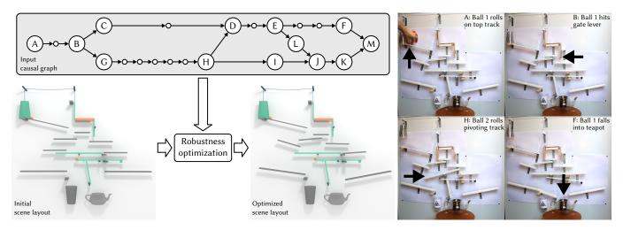
Fig. 1. Our system takes as input an initial scene layout associated with a causal graph of expected events. It then combines simulation, search and learning to build a success probability measure with respect to layout perturbations, and optimizes the layout for robustness against manual placement errors during assembly. The optimized layout is then exported as a guide sheet and used to successfully assemble complex chain reactions in the physical world.
