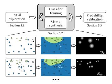
Fig. 8. **Building the SPD.** Top: main steps of our global SPD approximation method. Bottom: detail of the active learning loop: at iteration k, we use the current dataset X (left) to train an SVM (middle; classification shown as background colors). The new support vectors (black dots) are used to build a new distribution  $\mathcal{D}_k$  (right; probability density shown in white) that encourages additional sampling where the classifier is the most uncertain (i.e., near the boundary).
