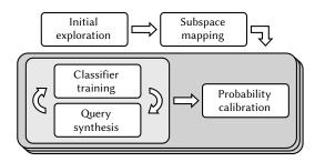
Fig. 10. **Extended SPD building pipeline.** We propose an extended version of our SPD building to scale with a high-dimensional design space.
