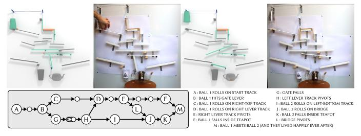
Fig. 14. TEAPOTADVENTURE scenario. See Figure 1 for initial layout. This figure shows rendered versus assembled layouts for start and end frames of the optimized layout. Ball 1 triggers the fall of the middle gate, releasing ball 2. Ball 2 hits the gate and takes the left route, falling on a lever so that ball 1 can roll underneath. Ball 2 then makes the central weight fall, liberating the bottom bridge. Both balls then meet in the teapot. Please see the supplementary video.
