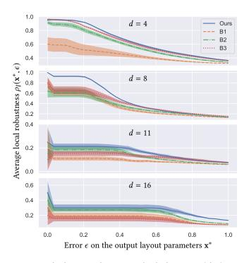
Fig. 15. Local robustness plots. Average local robustness  $\rho_l(\mathbf{x}^*, \epsilon)$  as a function of the error  $\epsilon$  on the layout parameters  $\mathbf{x}^*$  output by each method, for problems of different dimension d. Each curve is surrounded by a standard error of the mean interval (with T = 10 runs per method). Scenarios are respectively causalitySwitch, ballRun, longChain and teapotAdventure.
