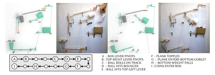
Fig. 13. **LONGCHAIN scenario.** A long chain of events that is triggered by the box weight pivoting an initial lever. Dominoes topple and send a ball onto a track to go hit a lever, which makes a plank topple through a narrow entrance into a goblet. This triggers the fall of the bottom weight, and in turn, the central goblet pivots to let coins fall into the box. Please refer to the supplementary video.
