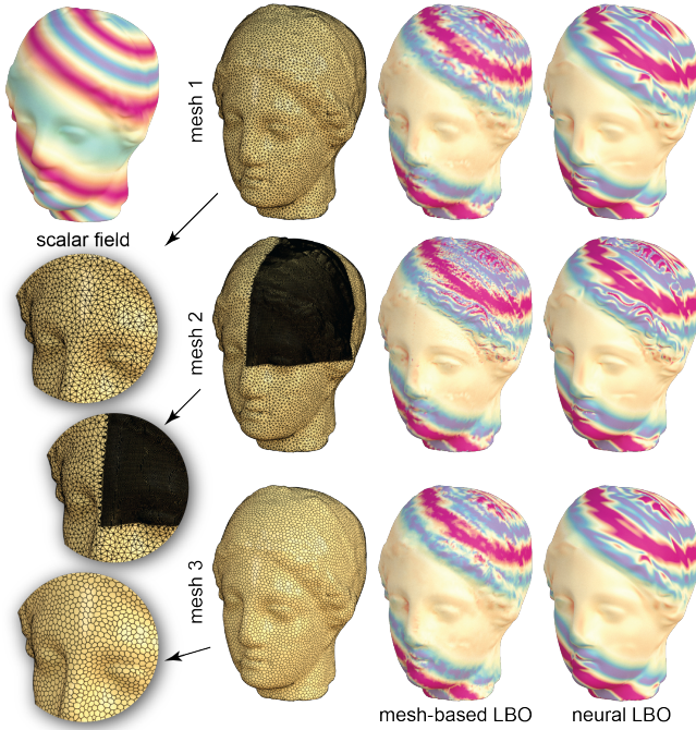
Figure 12: Robustness of Neural LBO (Non-Analytic). For non-analytic surfaces, we do not have access to a ground-truth LBO, because the precise underlying surface geometry is ambiguous. However, we show that the neural LBO is more consistent than mesh-based LBOs when fitted to different meshes of the same surface. This is because the smooth geometry of the SNS remains quite consistent when fitted to different meshes of the same surface, and the neural LBO is defined everywhere on the smooth surface - not just at the mesh-vertices. The neural LBO on mesh 2 does display some visible differences, however this is because the hair of Igea contains some high-frequency details. This is a signal which was lost in the lower-resolution meshes, so it is not an artefact or noise.
